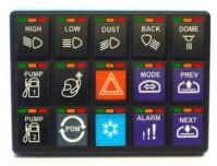
Each button has 3 indicators along the top. These lights report the status of a specific PDM Output for the function of that key.
